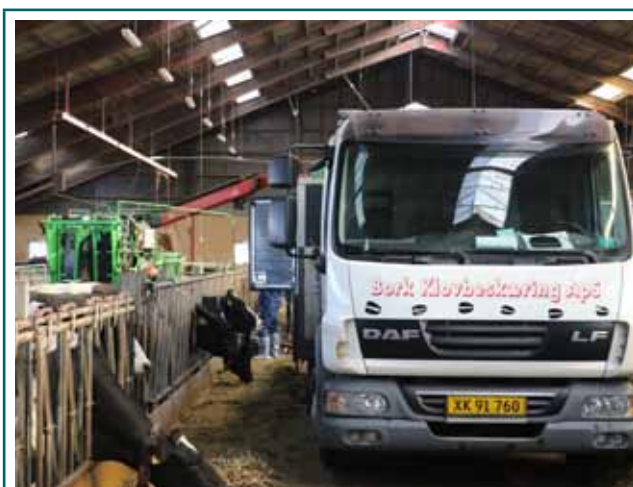
The truck on which the units is transported equipped with a crane to place the trimming unit amongst the cows
